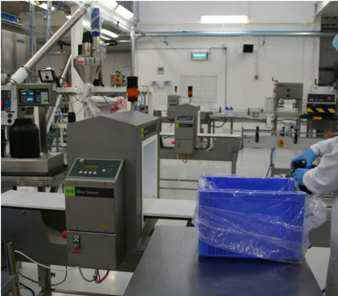
S+S UNICON Metal detection systems ensure end of line quality at Reflex Nutrition. (Photo: S+S)
